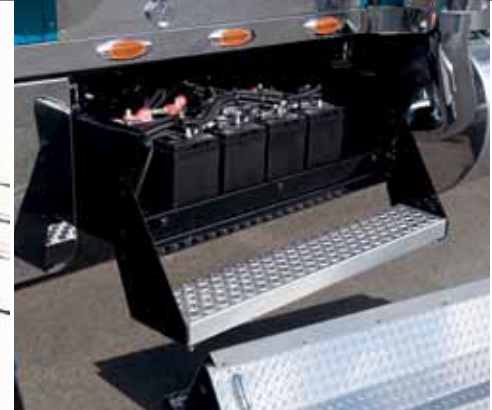
Here is another reason Kenworths are so dependable: 12-volt maintenance-free batteries, held firmly in place and mounted on the left-hand side, close to the starter motor for minimum voltage drop.
