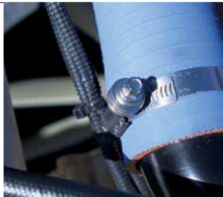
Constant torque hose clamps – standard on Kenworth trucks – go on tight and stay that way.
