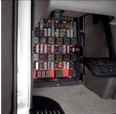
The T800's power distribution box puts all circuit protection elements – fuses, relays and breakers – in one quick-to-reach location.
