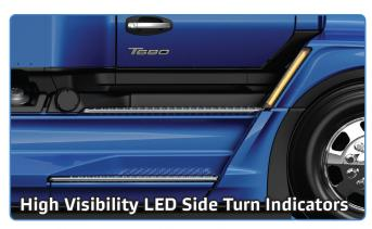
Unmistakable 17.3"-long LED side turn indicators, mounted to the trailing edge of the fender, greatly increase visibility for surrounding traffic. Redesigned steps allow for enhanced cab access.
