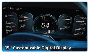
An industry-first at this size, the high definition 15-inch digital display contains all the information a driver needs to operate the truck – configurable for as much or as little content as they want.
