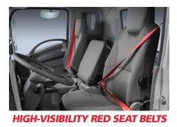
Red seat belts provide quick visual verification that seat belts are being worn to conform with safety regulations (front window seats only). (MY21 FTR shown)
