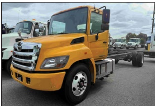
(3) 2019 HINO 338, 260 HP Hino Engine, Automatic Transmission, 33,000 GVW w/Air Suspension, 271" WB, 204" CA.
