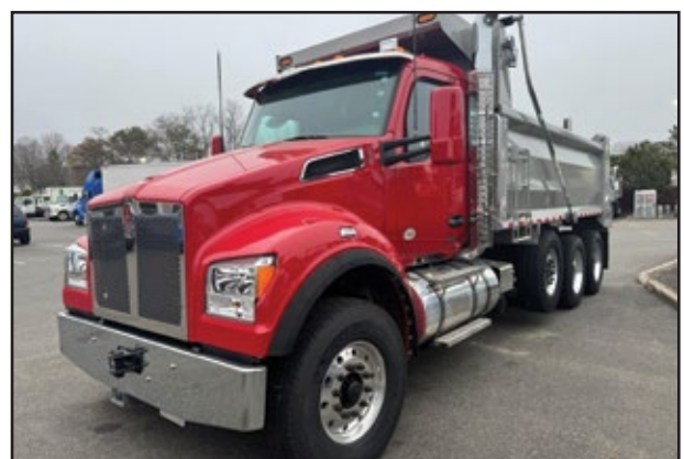
2024 KENWORTH T880s, 455 HP Paccar MX-13 Engine, 4500 RDS Transmission, 20,000 Front Axle, 46,000 Rear w/Air Suspension, Strbl Pshr, 18' Brandon Dump.
