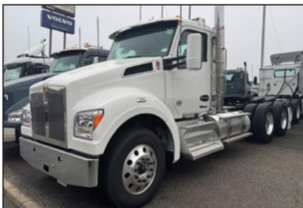
2025 KENWORTH T880s, 455 HP MX-13 Paccar Engine, PXDP-18F118D Transmission, 13,200 Front, 46,000 Rear w/Air Suspension. UNIT# NK-6793 Medford
