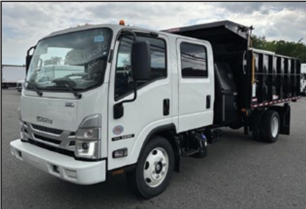
2024 ISUZU NRR Crew Cab, 215 HP Isuzu Diesel Engine, Automatic Transmission, 19,500 GVW, 12' Morgan Landscape Dump. UNIT# NH-0312 Monticello
