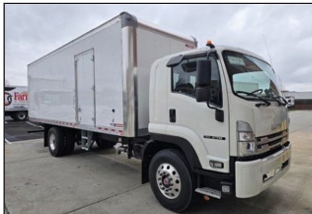
2025 ISUZU FTR, 260 HP Cummins B6.7 Engine, Allison Transmission, 25,950 GVW w/Air Suspension, 26' 97h x 196w Morgan Body.
