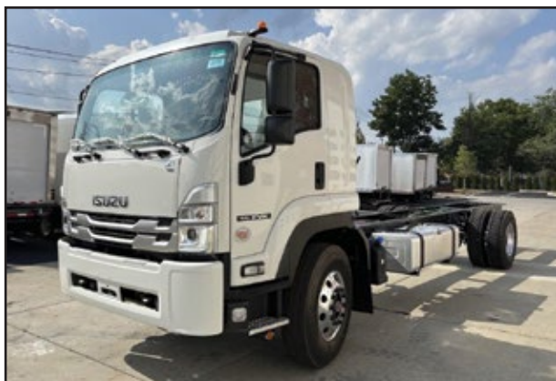
2025 ISUZU FVR LP, 260 HP Cummins B6.7 Engine, 2500 RDS Transmission, 33,000 GVW w/Spring Suspension, 224" WB, 199" CA.
