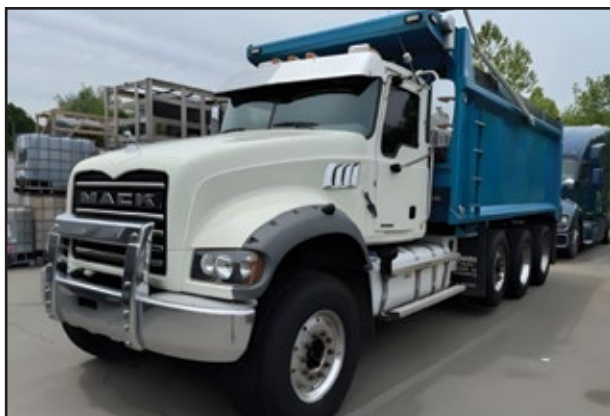
2022 MACK GR64F, 455 HP Mack MP8 Engine, Mack M-Drive Trans, 18,000 Front, 46,000 Rear w/Spring Susp, Pshr Axle, 17.6' Dump, 267,563 Miles. UNIT# YU-1111 Fairview.....$182,500
