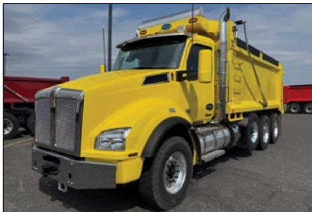
2025 KENWORTH T880, 510 HP Paccar MX13 Engine, 4500 RDS Transmission, 20,000 Front Axle, 46,000 Rear w/Spring Suspension, Strbl Pshr, 17.6' Heritage Dump. UNIT# RN-4139 Dayton
