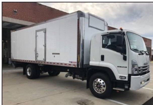
(2) 2025 ISUZU FVR, 260 HP Cummins B6.7 Engine, Allison Transmission, 33,000 GVW w/Air Suspension, 26' 96h x 97w Morgan Reefer Body w/Lift Gate.
