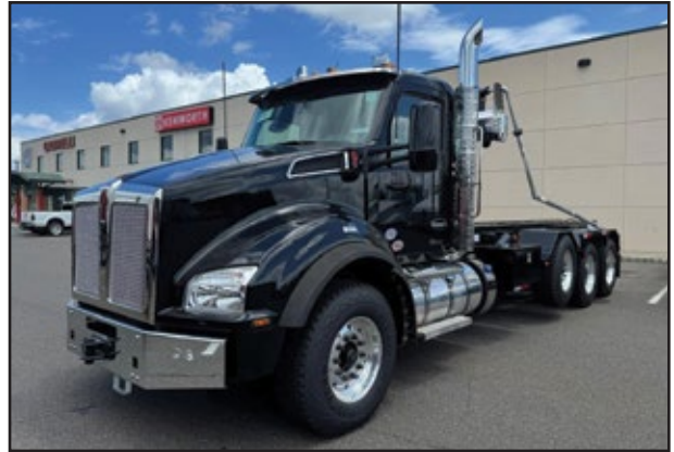
(4) 2026 KENWORTH T880, 500 HP Cummins X15 Engine, RTO16908LL 10 Spd, 20,000 Front Axle, 52,000 Rear w/Air Suspension, Strbl Pshr, 75k# American Roll Off. UNIT# RN-4218 Dayton, RN-4219 Ridgefield, RN-4221 Ridgefield, RN-4226 Ridgefield
