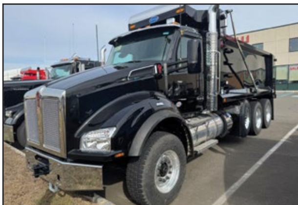
2025 KENWORTH T880, 510 HP Paccar MX-13 Engine, PXDP16F118D Automated Transmission, 20,000 Front Axle, 46,000 Rear w/Air Suspension, Strbl Pshr, 17.6' Heritage Dump. UNIT# RN-4085 Dayton
