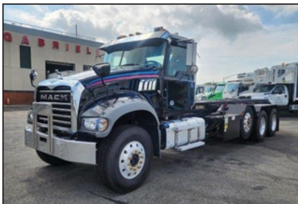
2019 MACK GU713, 455 HP Mack MP8 Engine, 4500 RDS Transmission, 20,000 Front, 46,000 Rear w/Spring Susp, Strbl Pshr, 75,000 Rudco Hoist, 154,005 Miles.
