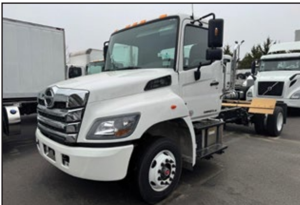
2025 HINO L6 ALP, 260 HP Cummins, 2200 RDS Trans., 25,500 GVW w/Air Suspension, 187" WB, 120" CA.
