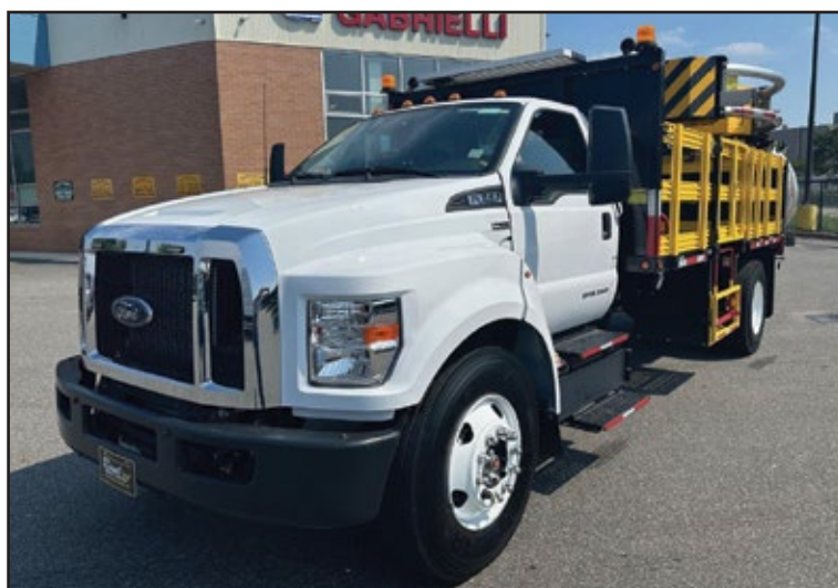
2024 FORD F750, 7.3L Gas Engine, Automatic Transmission, 25,999 GVW, 20' Knapheide Flatbed. UNIT# NF-8398 Milford
