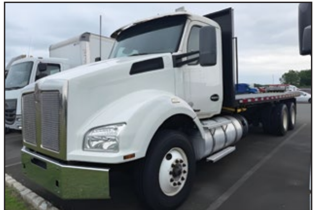
2016 KENWORTH T880, 405 HP Paccar MX13 Engine, Eaton FOM-14E310C-LAS Transmission, 14,600 Front, 46,000 Rear w/ Air Susp, 24' Flatbed, 190,002 Miles.
