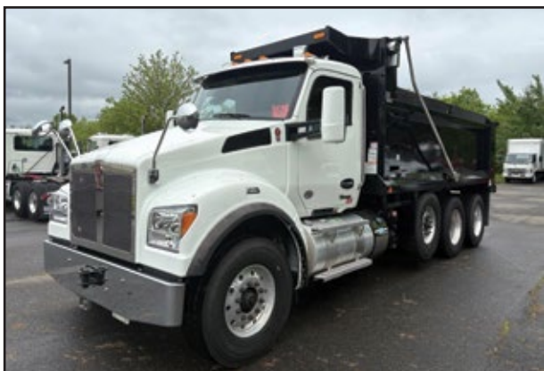
2023 KENWORTH T880s, 485 HP Paccar MX13 Engine, 4500 RDS Trans, 20,000 Front, 46,000 Rear w/Spring Susp, Strbl Pshr Axle, 17.6' Heritage Dump, 36,020 Miles. UNIT# UD-1782 Milford .....$228,500
