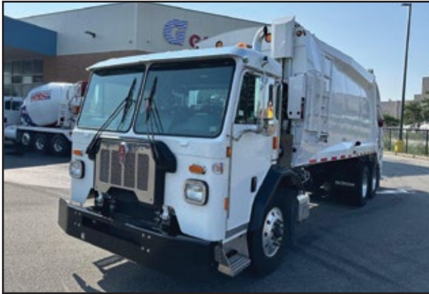
2024 KENWORTH L770, 400 HP Paccar MX-11 Engine, 4500 RDS Transmission, 20,000 Front Axle, 52,000 Rear w/Spring Suspension, 32 Yrd Rear Loader. UNIT# RN-3430 Eastern
