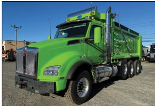
2025 KENWORTH T880, 565 HP Cummins X15 Engine, EXDP18F118D Transmission, 20,000 Front Axle, 46,000 Rear w/Spring Suspension, Strbl Pshr, 17.6' Heritage Dump. UNIT# RN-3895 Ridgefield
