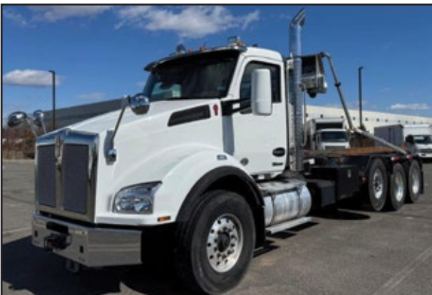
2023 KENWORTH T880, 485 HP Paccar MX13 Engine, 4500RDS Transmission, 20,000 Front, 46,000 Rear w/ Spring Susp, 75,000 Roll Off Hoist, 62,247 Miles. UNIT# UD-1760 Bloomsbury .....$225,500
