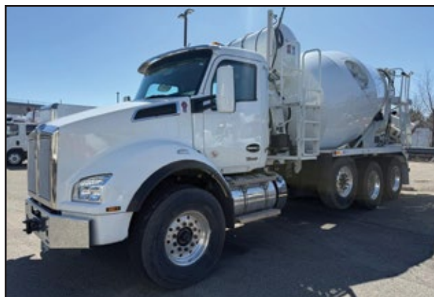
(3) 2025 KENWORTH T880, 430 HP Paccar MX-11 Engine, 4500 RDS Transmission, 20,000 Front Axle, 46,000 Rear w/ Spring Suspension, Strbl Pshr, 12 Yrd Continental Mixer.
