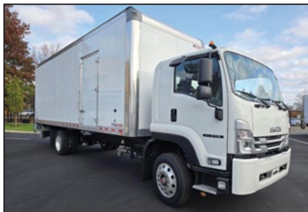
2025 ISUZU FTR LP, 260 HP Cummins B6.7 Engine, Allison Transmission, 25,950 GVW w/Air Suspension, 26' 103h x 102w Morgan Body w/Lift Gate.
