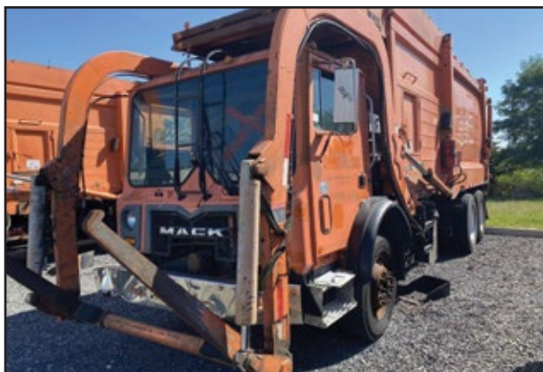
2015 MACK MRU613, 345 Mack MP7 Engine, 4500 RDS Automatic Transmission, 20,000 Front Axle, 58,000 Rear w/Spring Suspension, 40 Yrd. Heil Front End Loader.
