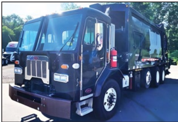
(2) 2017 PETERBILT 320, 320 Cummins Engine, 4500 RDS Automatic Transmission, 20,000 Front Axle, 46,000 Rear w/Spring Suspension, 28 Yrd. McNeilus Packer.
