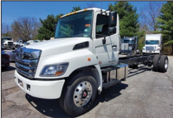
2026 HINO L6, 260 HP Cummins, 2500 RDS Transmission, 25,950 GVW w/Air Suspension, 271" WB, 203" CA.
