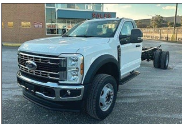
2024 FORD F600 4x4, 7.3L V8 Gas Engine, Automatic Transmission, 22,000 GVW, 205" WB, 120" CA.
