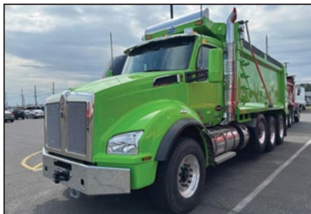
(3) 2025 KENWORTH T880, 565 HP Cummins X15 Engine, 4500 RDS Transmission, 20,000 Front Axle, 46,000 Rear w/ Spring Suspension, Strbl Pshr, 17.6' Heritage Dump. UNIT# RN-4161 Dayton, RN-4153 Dayton, RN-4162 Dayton
