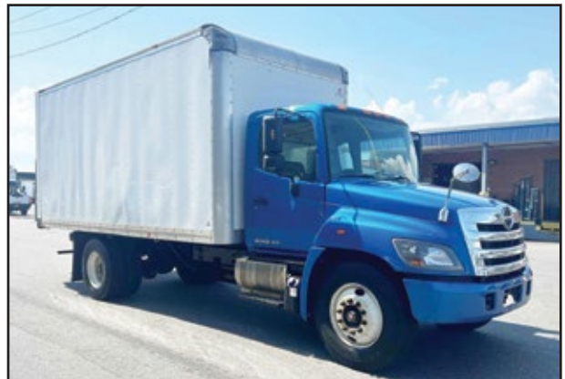
2018 HINO 268A, 230 HP Hino Engine, 2200 RDS Trans., 25,950 GVW w/Air Suspension, 18' 102h x 97w Supreme Body, 160,334 Miles.
