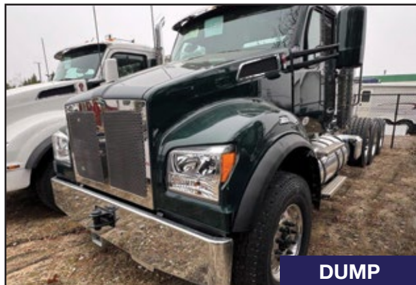
2025 KENWORTH T880s, 455 HP Paccar MX-13 Engine, 4500 RDS Transmission, 20,000 Front Axle, 46,000 Rear w/Spring Suspension, 244" WB, 158" CA. UNIT# NK-7204 Medford
