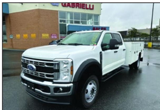
2024 FORD F450 Crew Cab 4x4, 7.3L Gas Engine, Automatic Transmission, 16,500 GVW, 11' Knapheide Service Body.
