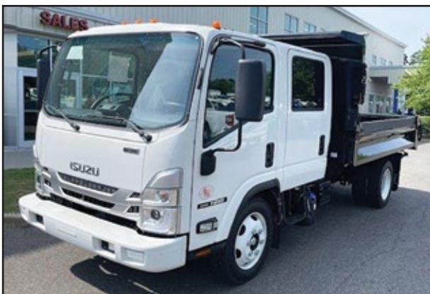
2024 ISUZU NRR Crew Cab, 215 HP Isuzu Diesel Engine, Automatic Transmission, 19,500 GVW, 11' Knapheide Dump.
