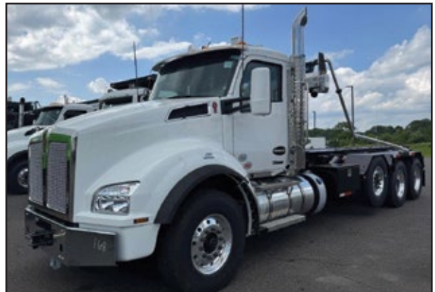
2025 KENWORTH T880, 500 HP Cummins X15 Engine, EXDP18F118D Transmission, 20,000 Front Axle, 46,000 Rear w/ Air Suspension, Strbl Pshr, 75k# American Roll Off. UNIT# DN-6014 Ridgefield Park
