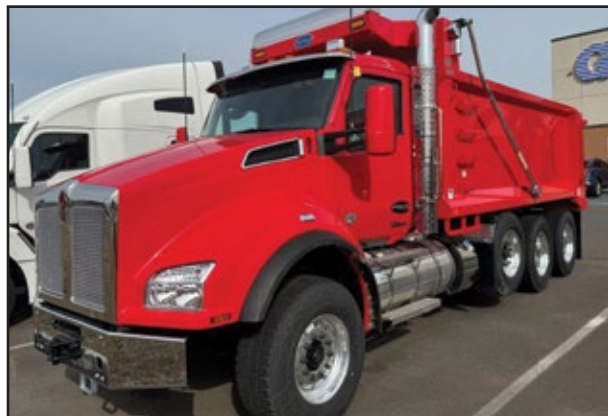
2025 KENWORTH T880s, 510 HP Paccar MX-13 Engine, PXDP16F118D Automated Transmission, 20,000 Front Axle, 46,000 Rear w/Air Suspension, Strbl Pshr, 17.6' Heritage Dump. UNIT# RN-4065 Dayton
