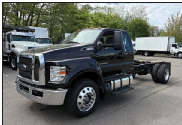
2026 FORD F650 Super Cab, 6.7L Diesel Engine, Automatic Transmission, 25,999 GVW, 203" WB, 108" CA.
