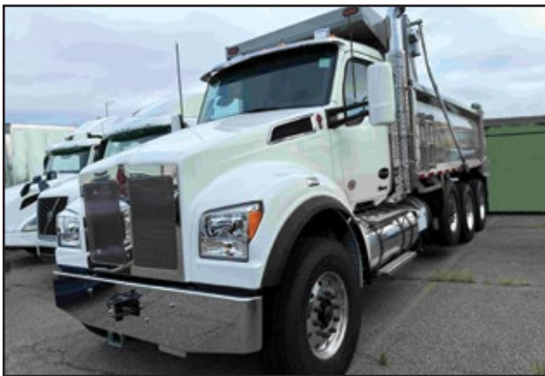
2025 KENWORTH T880s, 455 HP Paccar MX-13 Engine, 4500 RDS Transmission, 20,000 Front Axle, 46,000 Rear w/Spring Suspension, Strbl Pshr, 18' Brandon Dump.
