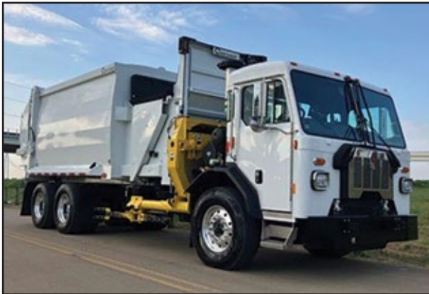
(3) 2024 KENWORTH L770, 400 HP Paccar MX-11 Engine, 4500 RDS Transmission, 20,000 Front Axle, 46,000 Rear w/ Spring Suspension, Curbtender 31 Yrd Power Pack. UNIT# RN-3981 Ridgefield, RN-3982 Enfield, RN-3983 Ridgefield
