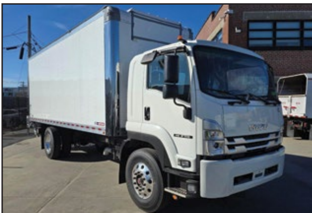
(8) 2024 ISUZU FTR, 260 HP Cummins B6.7 Engine, Allison Transmission, 25,950 GVW w/Air Suspension, 22' Morgan Reefer Body w/Lift Gate.
