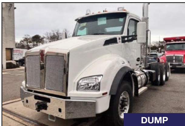
(3) 2025 KENWORTH T880, 500 HP Cummins X15 Engine, 4500 RDS Transmission, 20,000 Front Axle, 46,000 Rear w/ Spring Suspension, 232" WB, 156" CA. UNIT# NK-7179 Medford, NK-7180 Medford, NK-7181 Medford
