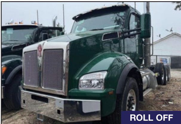
2025 KENWORTH T880, 455 HP MX13 Engine, 4500 RDS Transmission, 20,000 Front Axle, 46,000 Rear w/Air Suspension, Strbl Pshr, 262" WB, 194" CA. UNIT# NK-7203 Jamaica
