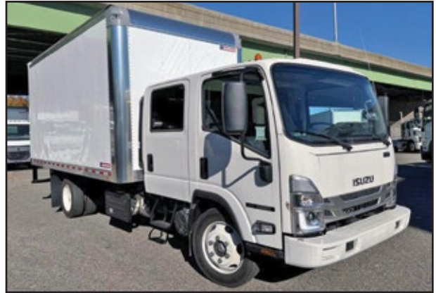
2024 ISUZU NRR Crew Cab, 215 HP Diesel Engine, Automatic Transmission, 19,500 GVW, 16' 91h x 96w Morgan Body.
