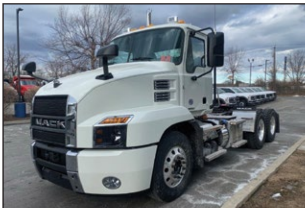
(4) 2026 MACK AN64T, 455 HP Mack MP8 Engine, M-Drive Transmission, 12,000 Front Axle, 40,000 Rear w/Air Suspension, 185" WB. UNIT# HM-1529 Milford, HM-1561 Bloomsbury, HM-1562 Bloomsbury
