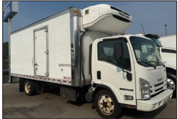
2017 ISUZU NRR, 215 HP Isuzu Engine, Aisin Transmission, 19,500 GVW, 18' 91h x 96w Morgan Reefer w/Thermo King Unit, 182,170 Miles.
