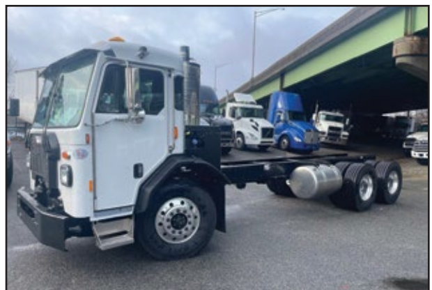
2025 KENWORTH L770, 400 HP Paccar MX-11 Engine, 4500 RDS Transmission, 20,000 Front Axle, 46,000 Rear w/Air Suspension, 215" WB.
