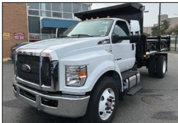
2025 FORD F650, 6.7L Diesel Engine, Automatic Transmission, 25,999 GVW, 14' Rugby Dump.
