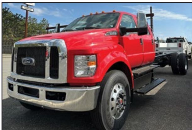
2024 FORD F750 Crew Cab, 7.3L Gas Engine, Automatic Transmission, 25,999 GVW, 266" WB, 156" CA.
