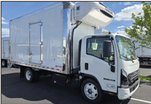
(3) 2025 ISUZU NRR, 215 HP Isuzu Diesel Engine, Automatic Transmission, 19,500 GVW, 16' 97h x 96w Morgan Reefer Body w/Thermo King Unit & Lift Gate.
