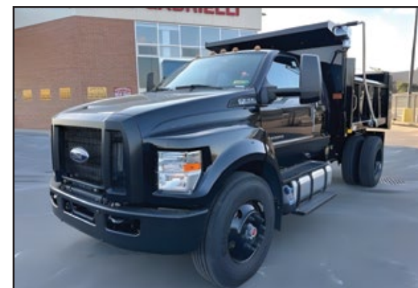
2025 FORD F750 Super Cab, 6.7L Diesel Engine, Automatic Transmission, 25,999 GVW, 10' Rugby Dump.
