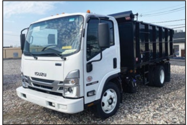
2024 ISUZU NRR, 215 HP Diesel Engine, Automatic Transmission, 19,500 GVW, 12' Galion Dump.
