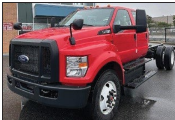
2026 FORD F750 Crew Cab, 7.3L Gas Engine, Automatic Transmission, 25,999 GVW, 212" WB, 102" CA.
