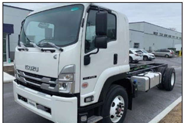
2025 ISUZU FVR LP, 260 HP Cummins B6.7 Engine, 2500 RDS Transmission, 33,000 GVW w/Spring Suspension, 188" WB, 163" CA.
