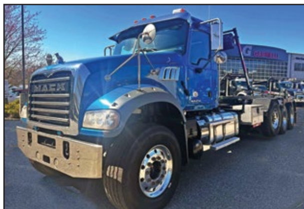
2018 MACK GU713, 505 HP Mack MP8 Engine, 18 Spd Transmission, 23,000 Front, 46,000 Rear w/Spring Susp, Pshr, 75,000 Roll Off, 190,299 Miles.
