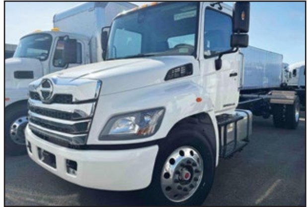
2025 HINO L6, 260 HP Cummins, 2200 HS Transmission, 25,950 GVW w/Air Suspension, 235" WB, 167" CA.
