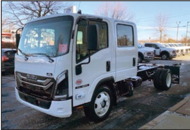
2025 ISUZU NRR Crew Cab, 215 HP Diesel Engine, Automatic Transmission, 19,500 GVW, 150" WB, 88" CA. UNIT# BI-1754 Milford
