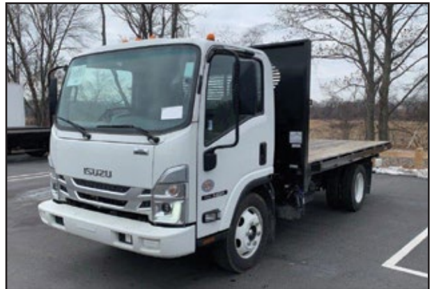
2023 ISUZU NQR, 215 HP Diesel Engine, Automatic Transmission, 17,950 GVW, 14' Wabash Flatbed Body.
