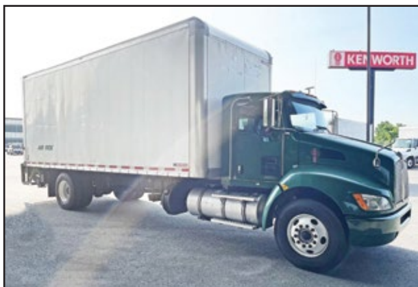
2016 KENWORTH T370, 280 HP Paccar PX-7 Engine, 2500 RDS Transmission, 33,000 GVW w/Spring Suspension, 24' 105h x 102w Supreme Body w/Lift Gate, 224,792 Miles. UNIT# UK-311 Enfield ..... $39,500
