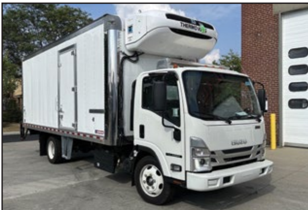
(3) 2024 ISUZU NQR, 215 HP Isuzu Diesel Engine, Automatic Transmission, 17,950 GVW, 20' 91h x 96w Morgan Reefer Body w/Thermo King Unit, w/Lift Gate.
