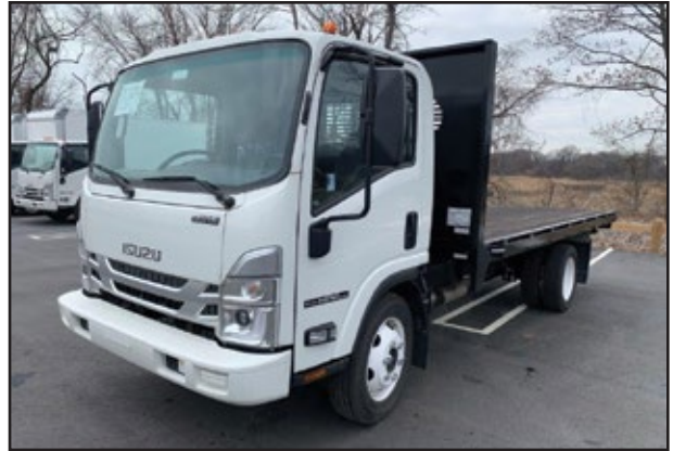
(2) 2024 ISUZU NPR HD, 6.6L 350 HP V8 Gas Engine, Automatic Transmission, 14,500 GVW, 16' Flatbed Body.
