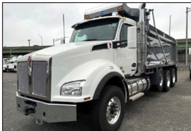
(2) 2025 KENWORTH T880, 525 HP Cummins X15 Engine, EXDP18F118D Transmission, 20,000 Front Axle, 46,000 Rear w/Spring Suspension, Strbl Pshr, 18' Heritage Dump. UNIT# NJ-12913 Jamaica, NJ-12920 Jamaica
