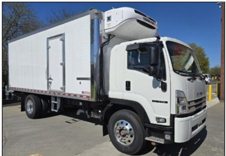
(2) 2024 ISUZU FTR, 260 HP Cummins B6.7 Engine, Allison Transmission, 25,950 GVW w/Air Suspension, 26' Morgan Reefer Body and Carrier Unit w/Lift Gate.
