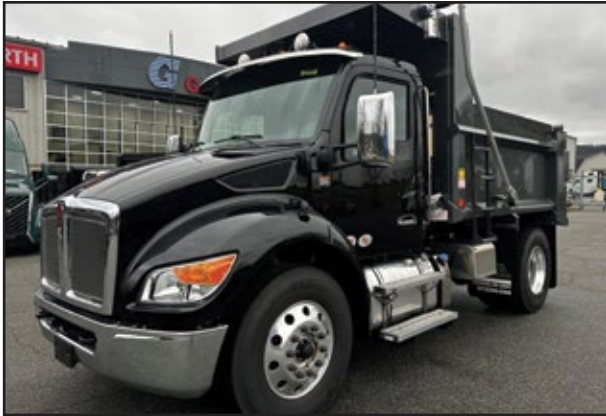
2025 KENWORTH T380, 330 HP PX-9 Engine, 3000 RDS Transmission, 33,000 GVW w/Spring Suspension, 10' TS Dump.
