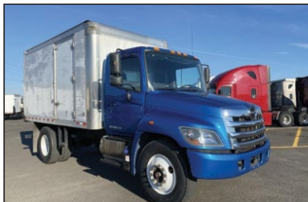
(4) 2018 HINO 268A, 230 HP Hino Engine, 2200 RDS Trans., 25,950 GVW w/Air Suspension, 14' 96h x 85w Supreme Body.
