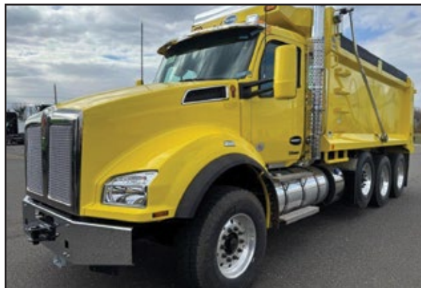
2025 KENWORTH T880, 510 HP Paccar MX13 Engine, TX-18 PXD-18F118D Transmission, 20,000 Front Axle, 46,000 Rear w/ Spring Suspension, Strbl Pshr, 17.6' Heritage Dump. UNIT# RN-4090 Dayton
