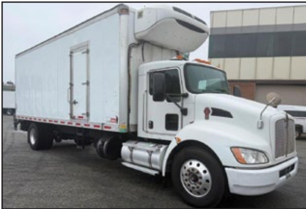
2014 KENWORTH T370, 270 HP Paccar PX-9 Engine, 3000 HS Transmission, 33,000 GVW w/Air Suspension, 24' 97hx102w Kidron Body w/Thermo King Unit & Lift Gate, 235,404 Miles.
