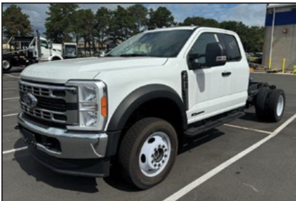
2023 FORD F550 4x4 Super Cab, 6.7L Diesel Engine, Automatic Transmission, 19,500 GVW, 168" WB, 60" CA.
