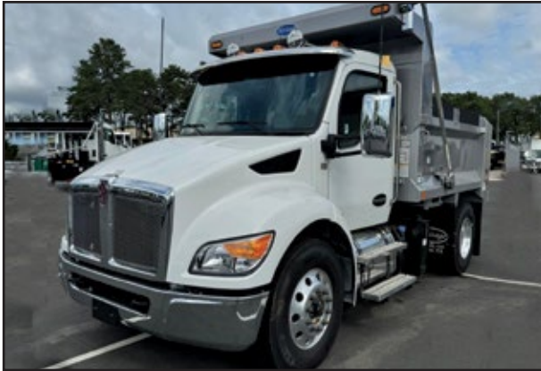
2025 KENWORTH T380, 330 HP PX-9 Engine, 3000 RDS Transmission, 33,000 GVW w/Spring Suspension, 10' Heritage Dump. UNIT# DN-4114 Medford
