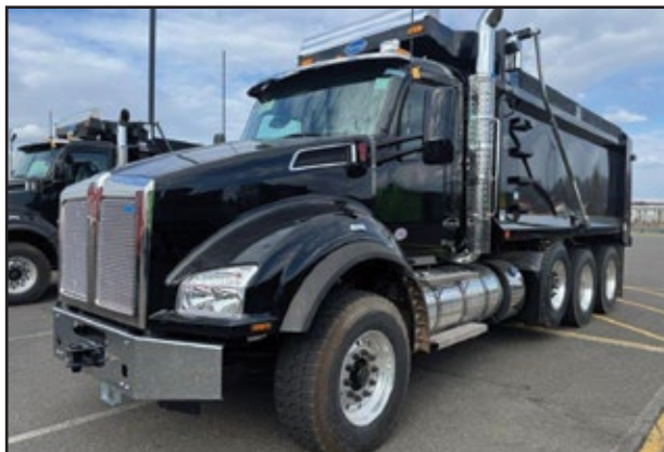
(2) 2025 KENWORTH T880, 510 HP Paccar MX13 Engine, TX-18 PXD-18F118D Transmission, 20,000 Front Axle, 46,000 Rear w/ Spring Suspension, Strbl Pshr, 17.6' Heritage Dump. UNIT# RN-4086 Dayton, RN-4087 Dayton
