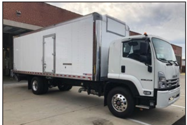
(2) 2025 ISUZU FVR, 260 HP Cummins B6.7 Engine, Allison Transmission, 33,000 GVW w/Air Suspension, 26' 96h x 97w Morgan Reefer Body w/Lift Gate.
