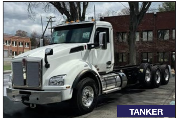
(3) 2026 KENWORTH T880, 525 HP Cummins X15 Engine, EXDP18F118D Transmission, 20,000 Front Axle, 46,000 Rear w/Spring Suspension, Strbl Pshr, 258" WB, 184" CA. UNIT# CK-1444 Enfield, CK-1477 Enfield, CK-1443 Enfield
