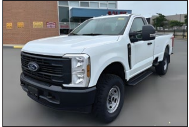
2025 FORD F250 Regular Cab 4x4, 6.8L Gasoline Engine, Automatic Transmission, 10,300 GVW, 8' Bed. UNIT# EF-1193 Eastern
