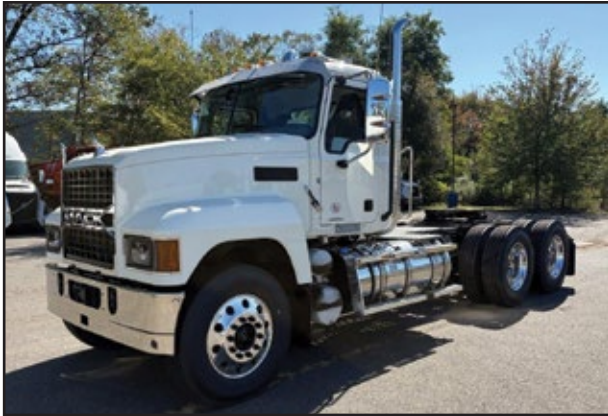
(2) 2026 MACK P164T, 5045 HP Mack MP8 Engine, M-Drive Trans., 14,600 Front Axle, 46,000 Rear w/Air Suspension, 213" WB. UNIT# NJ-13270 Montgomery , NJ-13289 Milford
