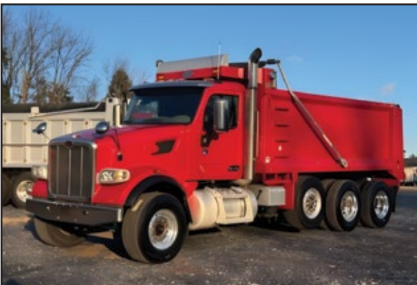
2020 PETERBILT 567, 505 HP Cummins X15 Engine, RTLO18918B Transmission, 20,000 Front, 46,000 Rear, Spring Suspension, Strbl Pshr, 17.5' Heritage Dump, 328,487 Miles. UNIT# CB-24P166T Coopersburg .....$147,500
