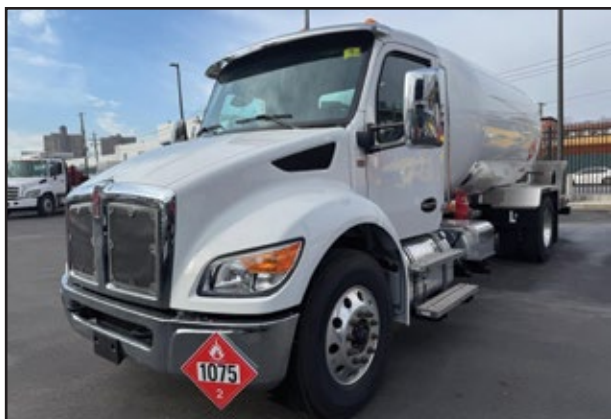
2025 KENWORTH T380, 330 HP PX-9 Engine, 3000 RDS Transmission, 33,000 GVW w/Air Suspension, Westmor Propane Tank.
