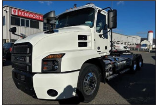
(15) 2026 MACK AN64T, 445 HP Mack MP8 Engine, M-Drive Transmission, 12,000 Front Axle, 40,000 Rear w/Air Suspension, 185" WB.
