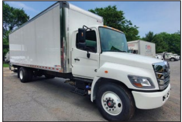
2026 HINO L7, 260 HP Cummins, 2500 RDS Transmission, 33,000 GVW w/Air Suspension, 26' 102h x 96w Morgan Body w/Lift Gate.
