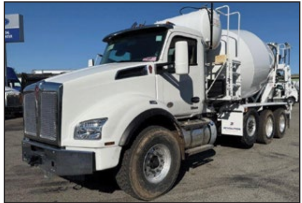
(5) 2025 KENWORTH T880, 430 HP Paccar MX-11 Engine, 4500 RDS Transmission, 20,000 Front Axle, 46,000 Rear w/Spring Suspension, Strbl Pshr, 12 Yrd Revolution Mixer. UNIT# DN-6079 Jamaica, DN-6068 Jamaica, DN-6075 Jamaica, DN-6080 Jamaica, DN-6081 Jamaica
