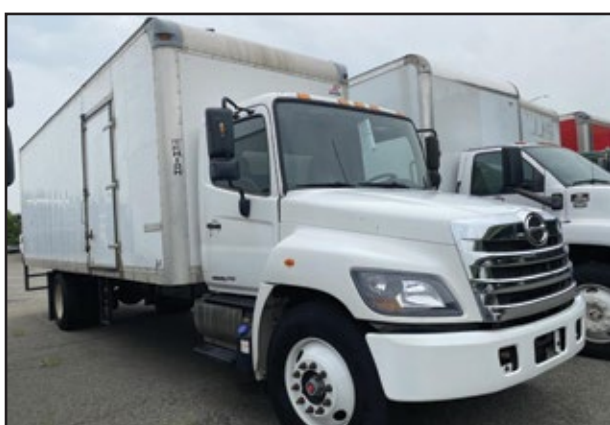
(3) 2016 HINO 338, 260 HP Hino Engine, Automatic Transmission, 33,000 GVW w/Spring Suspension, 26' 97h x 102w Supreme Body.
