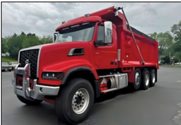
(2) 2025 VOLVO VHD84F, 455 HP Volvo D13 Engine, 4500 RDS Trans, 20,000 Front Axle, 46,000 Rear w/ Spring Suspension, Strbl Pshr, 17.6' Heritage Dump.
