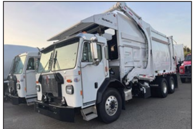
2024 KENWORTH L770, 400 HP Paccar MX-11 Engine, 4500 RDS Transmission, 20,000 Front Axle, 52,000 Rear w/Spring Suspension, McNeilus 32 Yrd Front End Loader. UNIT# RN-3416 Jamaica
