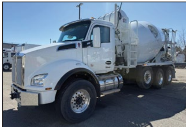
(3) 2025 KENWORTH T880, 430 HP Paccar MX-11 Engine, 4500 RDS Transmission, 20,000 Front Axle, 46,000 Rear w/ Spring Suspension, Strbl Pshr, 12 Yrd Continental Mixer. UNIT# NK-7147 Jamaica, NK-7160 Medford, NK-7135 Jamaica
