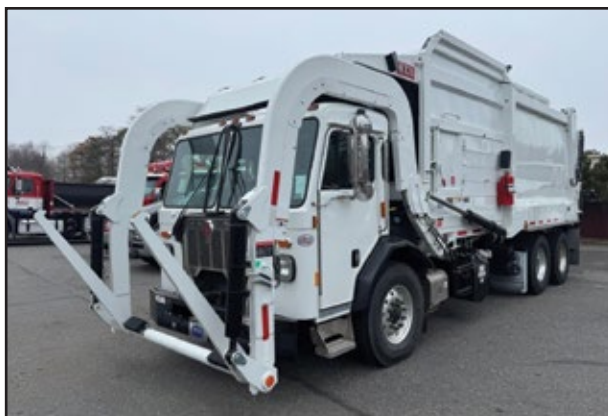
(4) 2025 KENWORTH L770, 400 HP Paccar MX-11 Engine, 4500 RDS Transmission, 20,000 Front Axle, 46,000 Rear w/ Spring Suspension, Heil 28 Yrd Front End Loader. UNIT# RN-3964, RN-4073 Medford, RN-4078 Bronx, RN-4079 Montgomery
