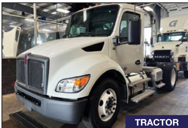
2025 KENWORTH T480, 330 HP PX-9 Engine, TX-12 PO16F112C Paccar Transmission, 12,500 Front Axle, 23,000 Rear w/Spring Suspension, 151" WB. UNIT# DN-4168 Dayton
