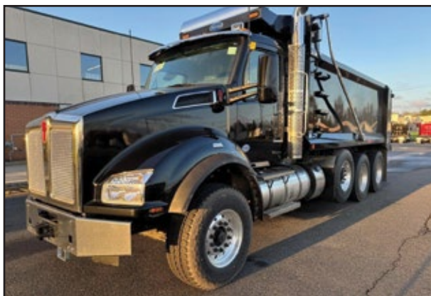
2025 KENWORTH T880, 510 HP Paccar MX13 Engine, TX-18 PXD-18F118D Transmission, 20,000 Front Axle, 46,000 Rear w/Spring Suspension, Strbl Pshr, 17.6' Heritage Dump. UNIT# RN-4137 Dayton
