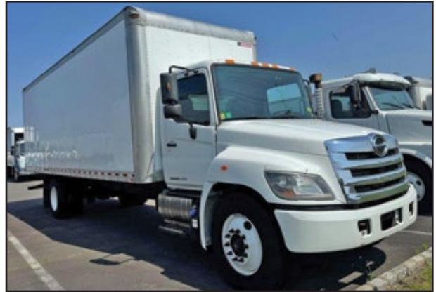
2018 HINO 268A, 230 HP Hino Engine, Automatic Transmission, 25,950 GVW w/Air Suspension, 26' 102h x 97w Morgan Body 108,128 Miles.
