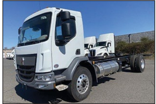
(3) 2025 KENWORTH K270, 260 HP PX-7 Engine, 2500 RDS Transmission, 26,000 GVW, Air Suspension, 218" WB, 206" CA. UNIT# DN-4104 Medford , DN-4158 Medford , DN-4153 Medford
