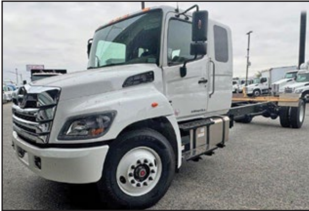
2025 HINO L6 Ext Cab, 260 HP Cummins, 2500 RDS Transmission, 25,950 GVW w/Air Suspension, 301" WB, 204" CA.
