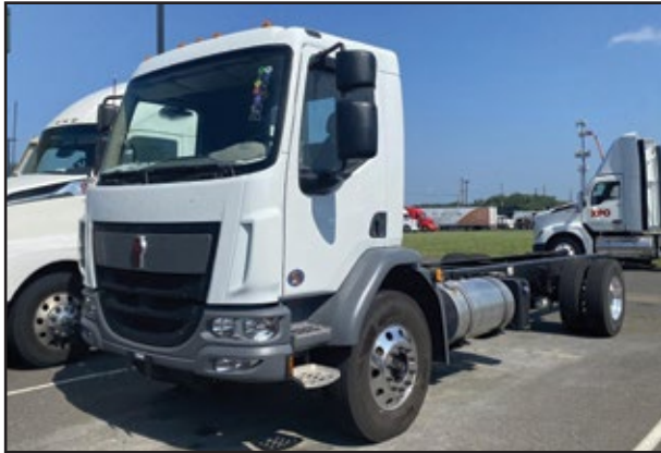
(2) 2024 KENWORTH K370, 260 HP PX-7 Engine, 3000 RDS Transmission, 33,000 GVW, Spring Suspension, 206" WB, 195" CA. UNIT# NK-6579 Dayton , DN-3226 Dayton
