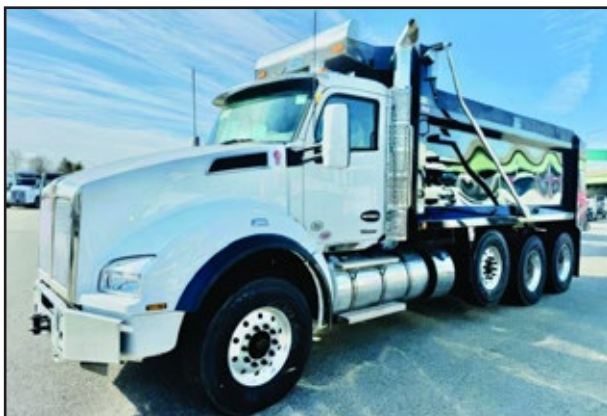
(3) 2025 KENWORTH T880, 525 HP Cummins X15 Engine, 4500 RDS Transmission, 20,000 Front Axle, 46,000 Rear w/ Spring Suspension, Strbl Pshr, 17.6' Heritage Dump. UNIT# NJ-13103 Jamaica, NJ-13101 Jamaica, NJ-13102 Jamaica
