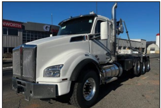
(2) 2025 KENWORTH T880, 500 HP Cummins X15 Engine, RTO16908LL 10 Spd, 20,000 Front Axle, 52,000 Rear w/Air Suspension, Strbl Pshr, 75k# American Roll Off. UNIT# RN-3805 Bloomsbury
