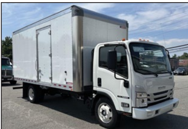
2025 ISUZU NRR, 6.6L 350 HP V8 Gas Engine, 1000 RDS Transmission, 19,500 GVW, 18' 91h x 96w Morgan Body.
