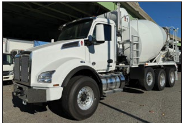
2026 KENWORTH T880, 430 HP Paccar MX-11 Engine, 4500 RDS Transmission, 20,000 Front Axle, 52,000 Rear w/Spring Suspension, Strbl Pshr, 12 Yrd Continental Mixer.
