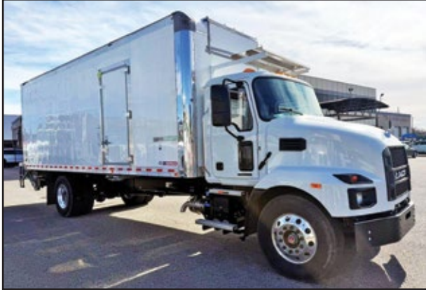
(2) 2025 MACK MD642, 260 HP Cummins ISB 6.7-260 D Engine, 2500 RDS Transmission, 25,995 GVW w/Air Suspension, 24' 97h x 96w Morgan Body w/Lift Gate. UNIT# NJ-12833 Jamaica, NJ-12878 Jamaica
