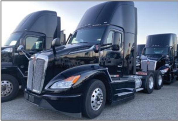
(11) 2024 KENWORTH T680, 455 HP MX-13 Paccar Engine, PO16F112C Transmission, 12,500 Front Axle, 40,000 Rear w/Air Suspension, 181" WB.
