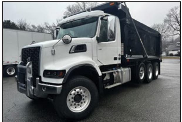
2025 VOLVO VHD84F, 500 HP Volvo D13 Engine, I-Shift Transmission, 20,000 Front Axle, 46,000 Rear w/Spring Suspension, Strbl Pshr, 17.6' Heritage Dump. UNIT# YV-1162 Bloomsbury
