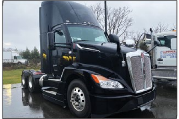
2024 KENWORTH T680, 450 HP X-15 Cummins Engine, EEO17F112 Transmission, 12,500 Front Axle, 40,000 Rear w/Air Suspension, 185" WB.
