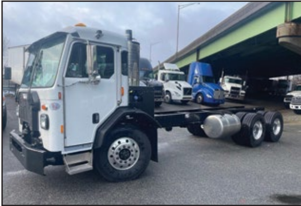
(2) 2025 KENWORTH L770, 400 HP Paccar MX-11 Engine, 4500 RDS Transmission, 20,000 Front Axle, 46,000 Rear w/Air Suspension, 215" WB. UNIT# RN-4037 Jamaica, RN-4072 Fairview
