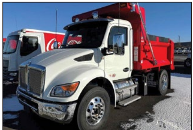
2025 KENWORTH T380, 330 HP PX-9 Engine, 3000 RDS Transmission, 33,000 GVW w/Spring Suspension, 10' Heritage Dump.
