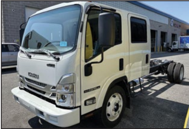
2024 ISUZU NPR HD Crew Cab, 6.6L 350 HP V8 Gas Engine, Automatic Transmission, 14,500 GVW, 176" WB, 115" CA.
