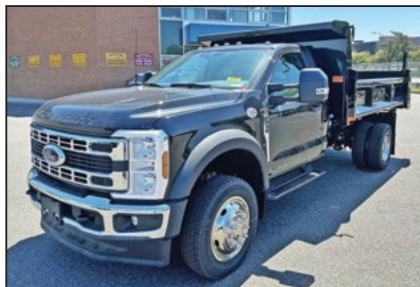
2024 FORD F550 4x4, 6.7L Diesel Engine, Automatic Transmission, 19,500 GVW, 11' Rugby Dump. UNIT# EF-1100 Bronx
