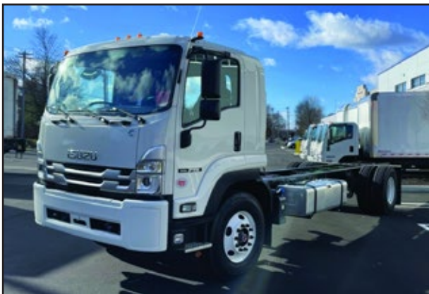
2025 ISUZU FTR, 260 HP Cummins B6.7 Engine, Allison Transmission, 25,950 GVW w/AirRide Suspension, 224" WB, 199" CA.
