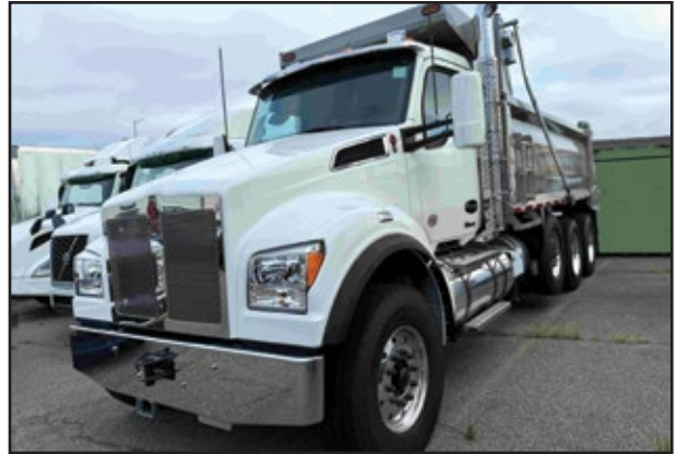
(3) 2025 KENWORTH T880s, 455 HP Paccar MX-13 Engine, 4500 RDS Transmission, 20,000 Front Axle, 46,000 Rear w/Air Suspension, Strbl Pshr, 18' Brandon Dump. UNIT# DN-4137 Jamaica, DN-4138 Eastern, DN-4156 Jamaica
