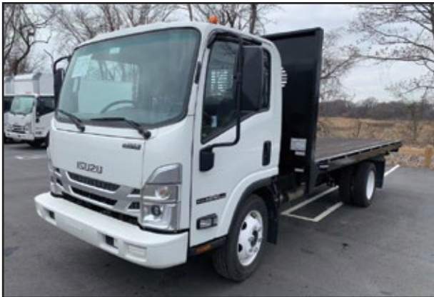
(2) 2024 ISUZU NPR HD, 6.6L 350 HP V8 Gas Engine, Automatic Transmission, 14,500 GVW, 16' Flatbed Body. UNIT# BI-1757 Milford, BI-1761 Milford
