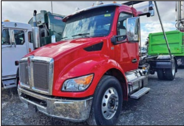
2025 KENWORTH T280, 330 HP PX-9 Engine, 3000 RDS Transmission, 26,000 GVW w/Spring Suspension, Ampliroll AL100S-15 Hooklift.
