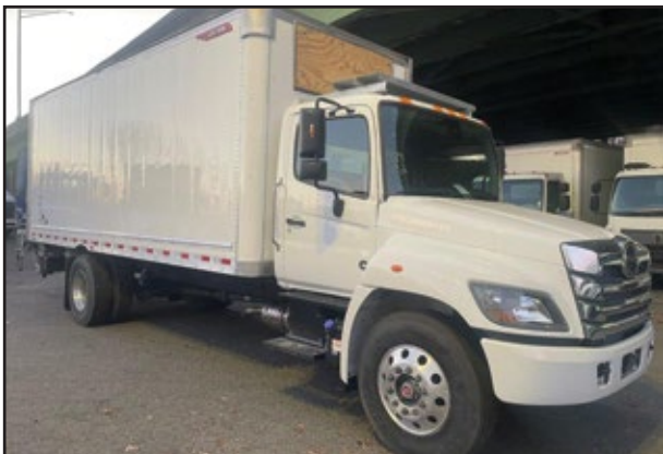
(3) 2025 HINO L6, 260 HP Cummins, 2500 RDS Trans., 25,950 GVW w/Air Suspension, 22' 101h x 96w Great Dane Reefer Body w/Lift Gate.
