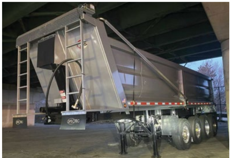
2023 SPECTOR ROCKETT DUMP, 30' Long x 96" Wide, 54" Sides, AR450, Heated Body, Double Acting Tailgate. UNIT# SRDD305496 Jamaica
