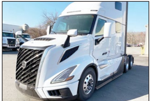
(13) 2025 VOLVO VNL64T660, 455 HP D-13 Volvo Engine, I-Shift Transmission, 12,000 Front Axle, 40,000 Rear w/Air Susp., 211" WB, 62" Double Bunk Sleeper.
