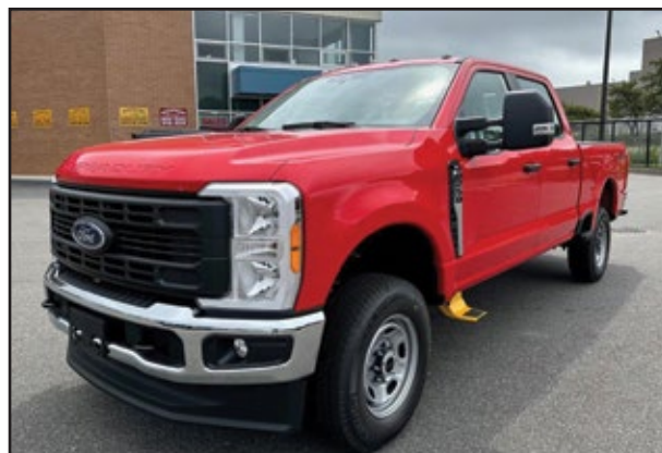
2023 FORD F250 Crew Cab 4x4, 6.8L Gas Engine, Automatic Transmission, 10,000 GVW, 6.75' Bed.
