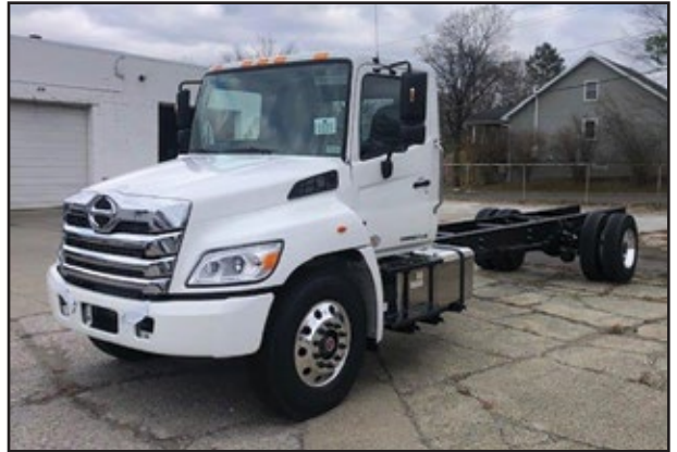
2025 HINO L6, 260 HP Cummins, 2500 RDS Transmission, 25,950 GVW w/Spring Suspension, 271" WB, 203" CA.
