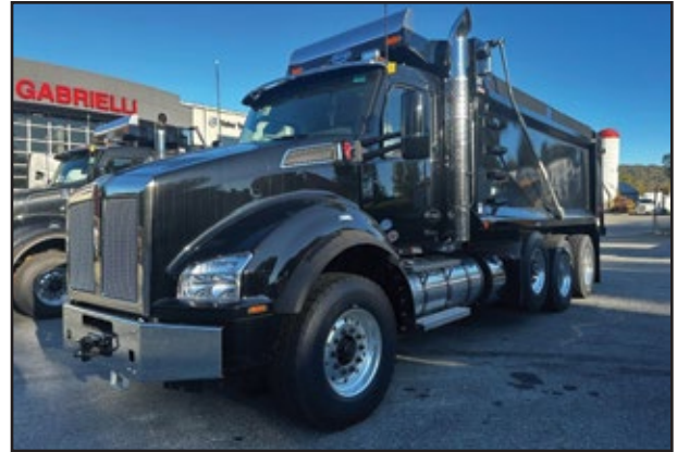
(4) 2025 KENWORTH T880, 565 HP Cummins X15 Engine, EXDP18F118D Transmission, 20,000 Front Axle, 46,000 Rear w/Spring Suspension, Strbl Pshr, 17.6' Heritage Dump. UNIT# RN-3845 Bloomsbury, RN-3841 Bloomsbury, RN-3935 Bloomsbury, RN-3831 Ridgefield
