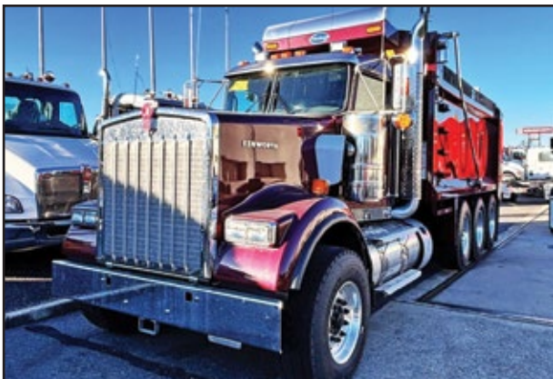
2025 KENWORTH W900, 565 HP Cummins X15 Engine, RTL020918B Transmission, 20,000 Front Axle, 40,000 Rear w/Air Suspension, Strbl Pshr, 17.6 Heritage Dump. UNIT# RN-3879 Medford
