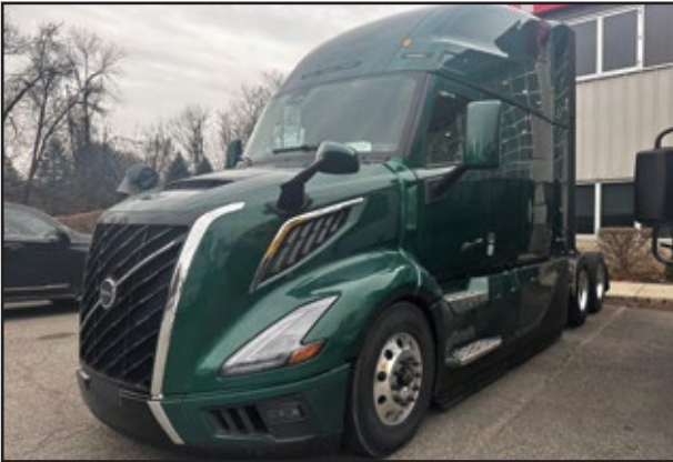
(4) 2025 VOLVO VNL64T860, 455 HP D-13 Volvo Engine, I-Shift Transmission, 13,200 Front Axle, 40,000 Rear w/Air Susp., 222" WB, 77" Double Bunk Sleeper. UNIT# NJ-13086 Jamaica, VY-1258 Bloomsbury, YV-1273 Bloomsbury, NJ-13175 Jamaica
