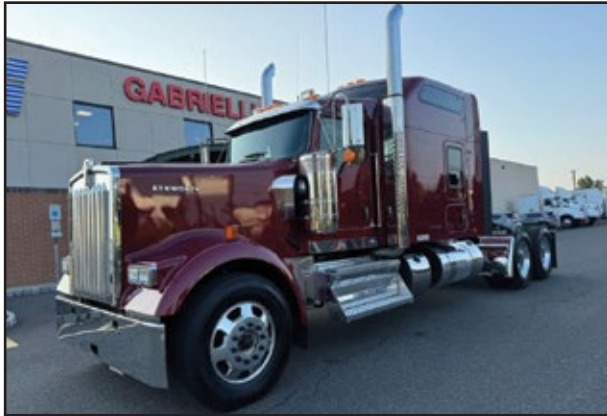
(2) 2025 KENWORTH W900L, 605 HP Cummins X15 Engine, RTL020918B Transmission, 13,200 Front, 40,000 Rear w/Air Susp, High Roof Sleeper. UNIT# DN-4172 Monticello, DN-6064 Dayton
