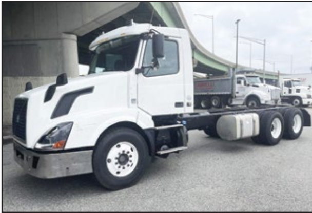
(2) 2017 VOLVO VNL, 405 HP D11 Engine, 10 Spd Manual Transmission, 16,000 Front Axle, 40,000 Rear Axle w/Air Suspension, 223 WB, 156" CA. UNIT# UD-1454 Jamaica 361,026 Miles..... $57,500 UNIT# UD-1455 Dayton 284,189 Miles..... $61,800
