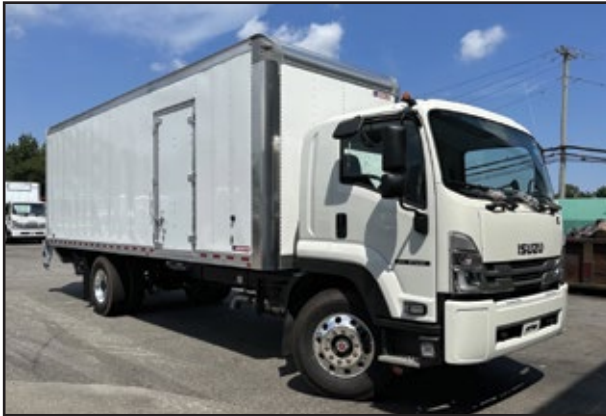
2025 ISUZU FVR, 260 HP Cummins B6.7 Engine, Allison Transmission, 33,000 GVW w/Air Suspension, 26' 96h x 97w Morgan Body w/Lift Gate.
