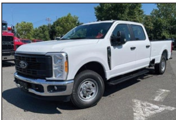
2023 FORD F350 Crew Cab, 6.8L Gas Engine, Automatic Transmission, 10,900 GVW, 8' Bed.
