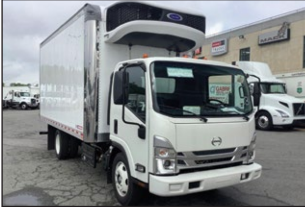
(2) 2024 HINO S5-COE, 215 HP Diesel Engine, Automatic Transmission, 19,500 GVW, 16' Morgan Reefer Body with Carrier Unit.
