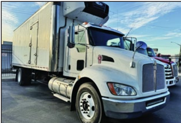
2019 KENWORTH T270, 280 HP Paccar PX-7 Engine, 2500 RDS Transmission, 26,000 GVW w/Spring Suspension, 24' 97hx96w Morgan Body w/Carrier Unit & Lift Gate, 123,257 Miles.
