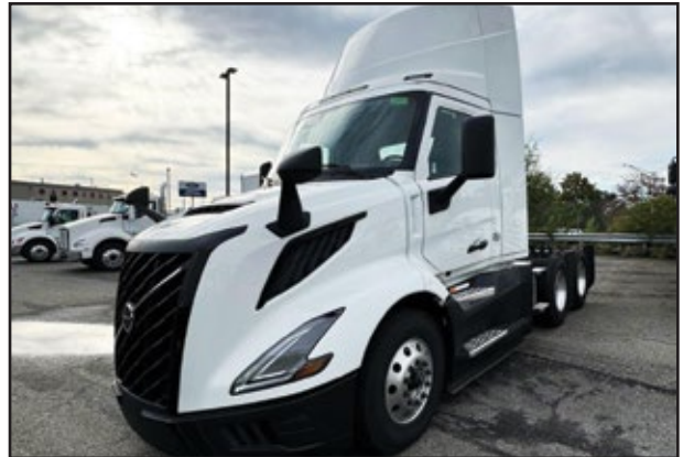
(5) 2025 VOLVO VNL64T300, 455 HP D-13 Volvo Engine, I-Shift Transmission, 12,500 Front Axle, 40,000 Rear w/Air Susp., 171" WB.
