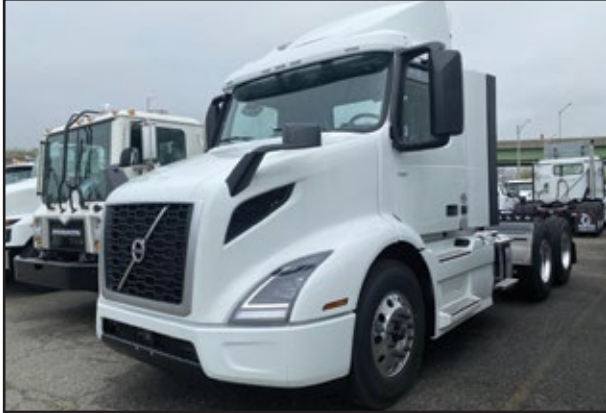
2025 VOLVO VNR64T300, 425 HP D-13 Volvo Engine, I-Shift Transmission, 12,000 Front Axle, 40,000 Rear w/Air Susp., 183" WB.
