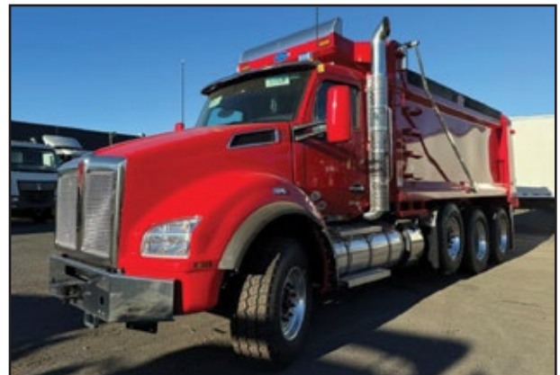
2025 KENWORTH T880, 565 HP Cummins X15 Engine, EXDP18F118D Transmission, 20,000 Front Axle, 46,000 Rear w/Spring Suspension, Strbl Pshr, 17.6' Heritage Dump. UNIT# RN-3816 Ridgefield
