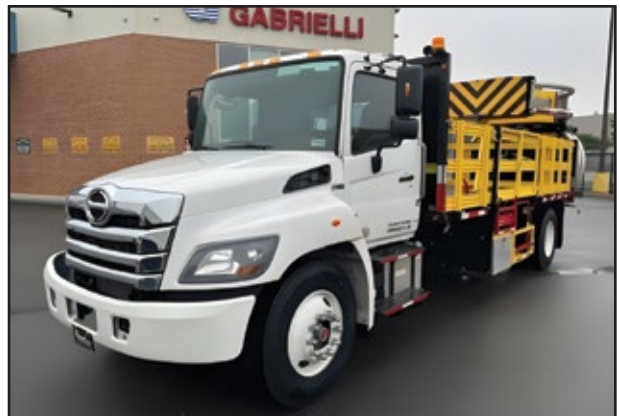
(5) 2025 HINO L6, 260 HP Cummins, 2500 RDS Transmission, 25,950 GVW w/Air Suspension, 18' Scorpion Attenuator Body.
