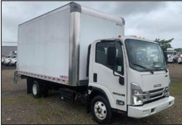
2023 ISUZU NQR, 215 HP Isuzu Diesel Engine, Automatic Transmission, 17,950 GVW, 18' 90h x 96w Utilimaster w/Lift Gate.
