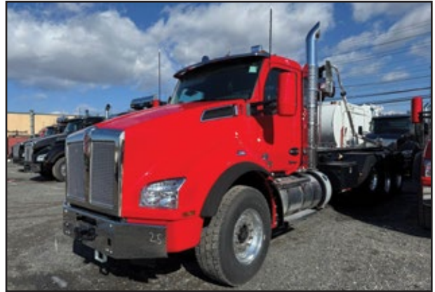
(2) 2025 KENWORTH T880, 500 HP Cummins X15 Engine, RTO16908LL 10 Spd, 20,000 Front Axle, 52,000 Rear w/Air Suspension, Strbl Pshr, 75k# American Roll Off. UNIT# RN-3803 Ridgefield, RN-3679 Ridgefield Park
