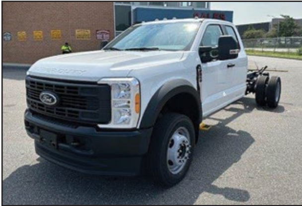
2024 FORD F550 4x4 Super Cab, 7.3L V8 Gas Engine, Automatic Transmission, 18,000 GVW, 192" WB, 84" CA. UNIT# EF-1123 Eastern
