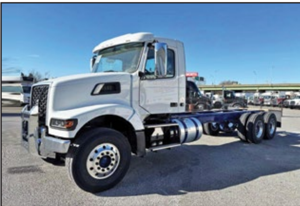
(2) 2025 VOLVO VHD84F, 425 HP Volvo D13 Engine, 4500 RDS Transmission, 20,800 Front Axle, 58,000 Rear w/Spring Suspension, 275" WB. UNIT# NJ-13169 Jamaica, NJ-13149 Jamaica
