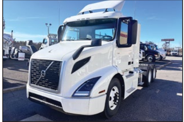
(2) 2025 VOLVO VNR64T300, 425 HP D-13 Volvo Engine, I-Shift Transmission, 12,000 Front Axle, 40,000 Rear w/Air Susp., 185" WB.
