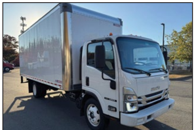
2024 ISUZU NRR, 6.6L 350 HP V8 Gas Engine, 1000 RDS Transmission, 19,500 GVW, 18' 91h x 96w Utilimaster Body.
