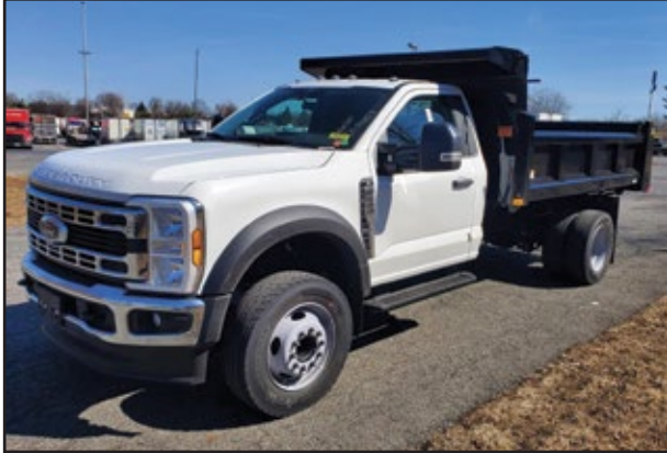
2024 FORD F600, 7.3L Gas Engine, Automatic Transmission, 22,000 GVW, 11' Rugby Dump Body. UNIT# EF-1149 Montgomery
