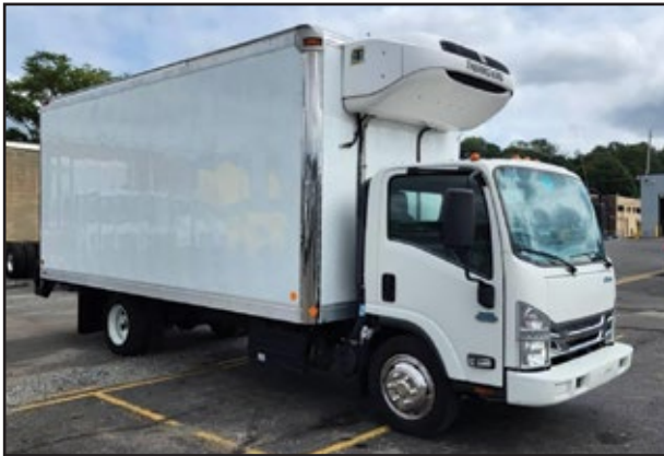
(2) 2022 ISUZU NRR, 215 HP Isuzu Engine, Aisin Transmission, 19,500 GVW, 18' Reefer Body w/Thermo King Unit & Lift Gate.
