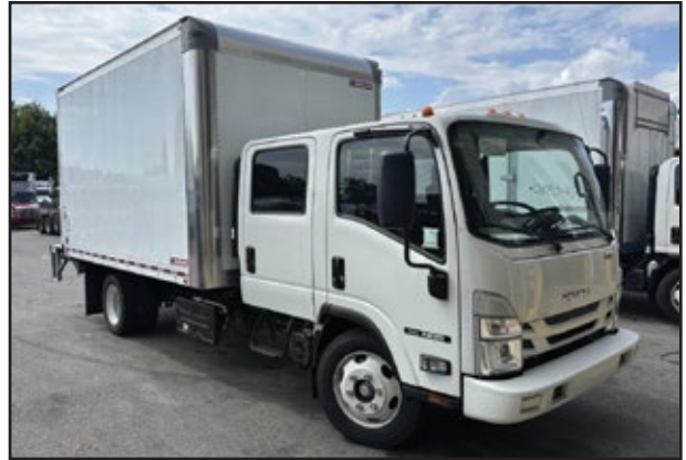
2024 ISUZU NRR Crew Cab, 215 HP Diesel Engine, Automatic Transmission, 19,500 GVW, 14' 91h x 96w Morgan Body w/Lift Gate.
