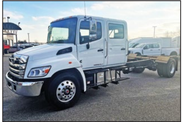
(2) 2025 HINO L7 Crew Cab, 260 HP Cummins, 2500 RDS Transmission, 25,950 GVW w/Air Suspension, 253" WB, 140" CA.
